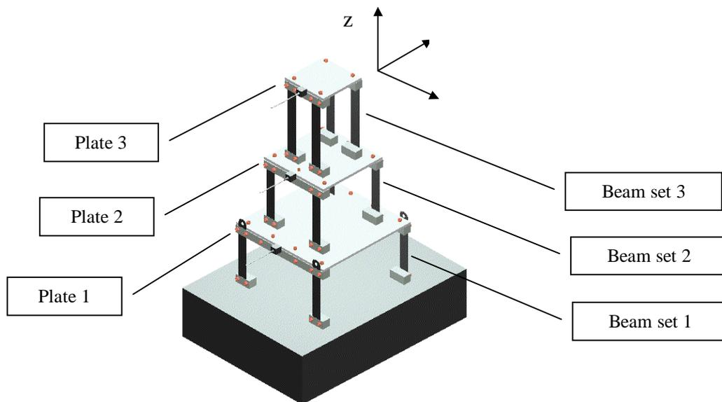
Figure 1. Mechanical system used in the experiments.
