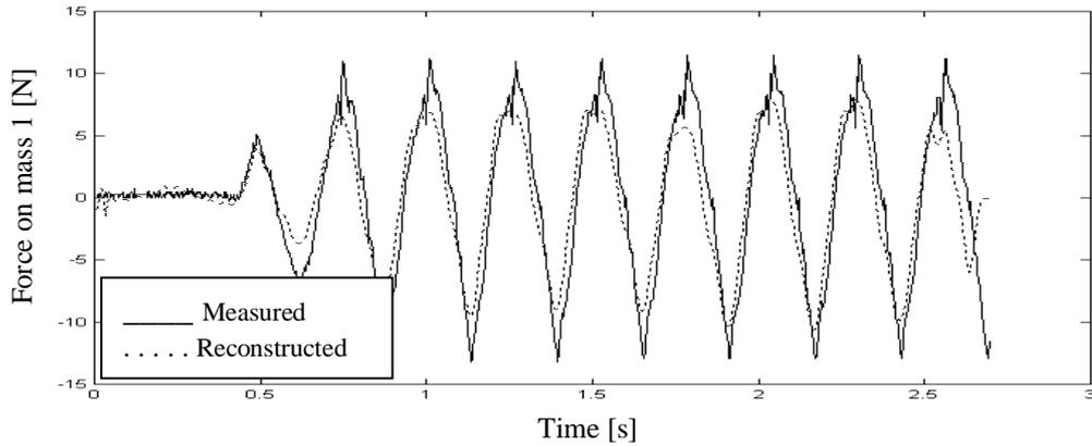
Figure 4. Measured and identified triangular forces at coordinate 1.
