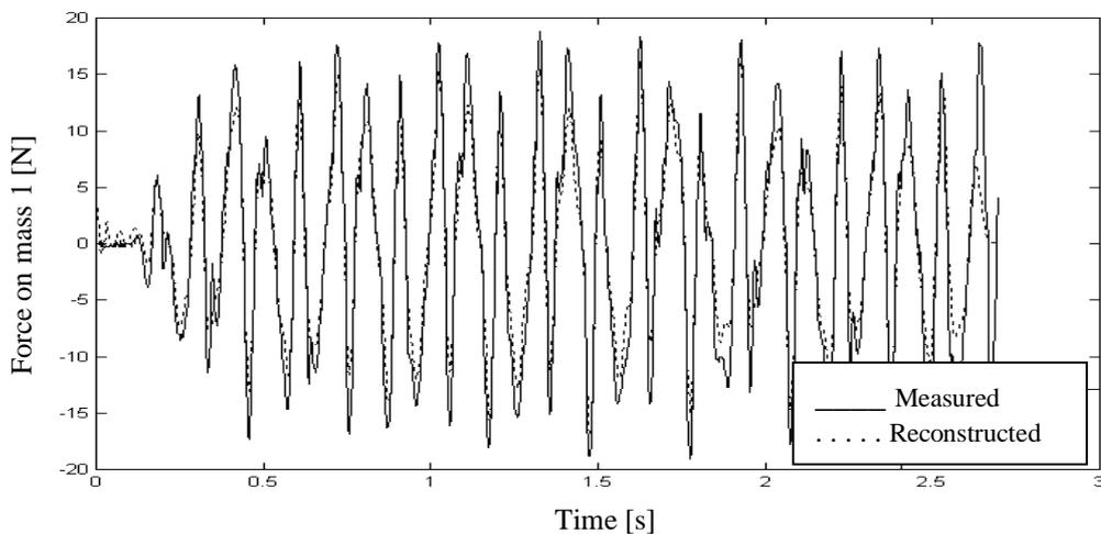
Figure 5. Measured and identified triangular forces at coordinate 1.
