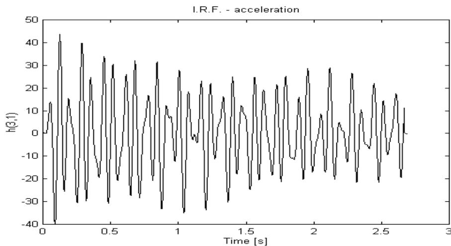
Figure 2 - IRF  $h_{31}(t)$  of the test-structure.
