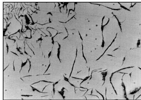
Figure 2: Optical image of gray cast iron plates graphites (200x).
