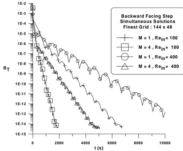
Figure 6 – Residue history for simultaneous solution with different number of grids and  $Re_{in}$  - V-cycle.
