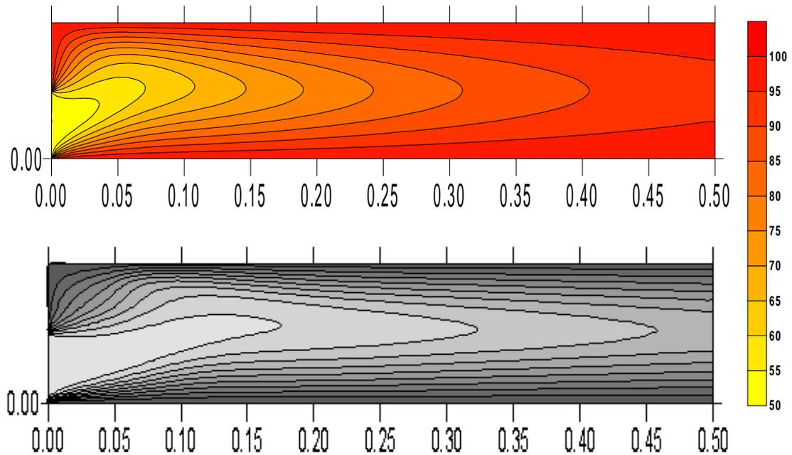
Figure 5 - Effect of  $Re_{in}$  on temperature pattern for backward facing step of Figure 1. From top to bottom:  $Re_{in}=100, 400$ .
