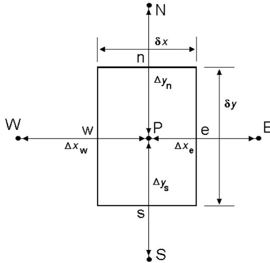
Figure 3 Control volume for discretization.
