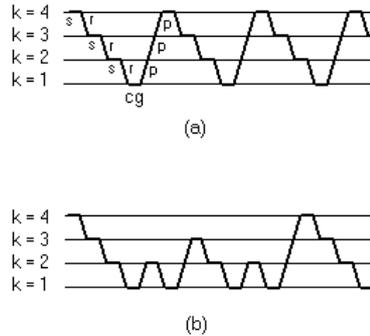
Figure 4 - Sequence of operations in a 4-grid iteration: (a) V-cycle; (b) W-cycle.
