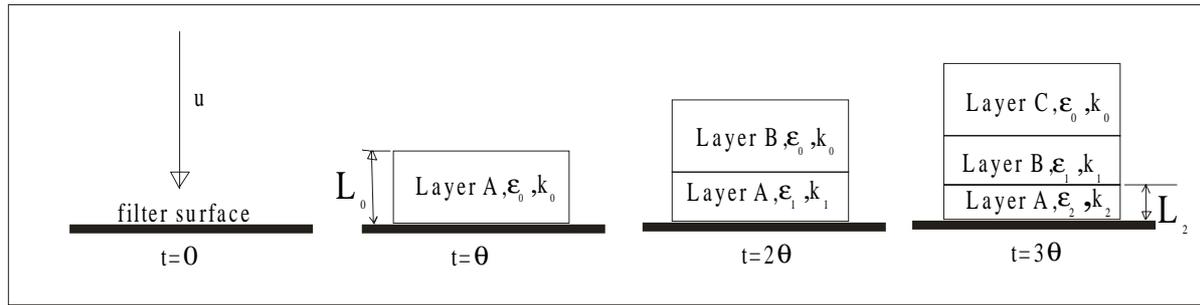
Figure 2. Schematic representation of the cake formation model
