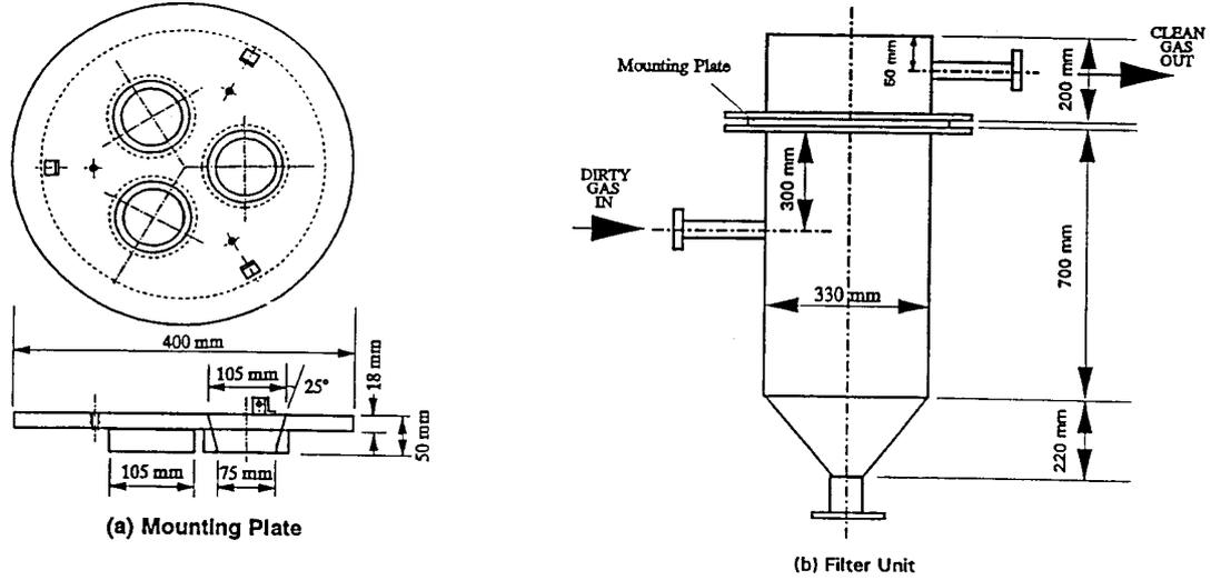
Figure 3 – Experimental filtration vessel used by Ergünder *et al.*(1997)
