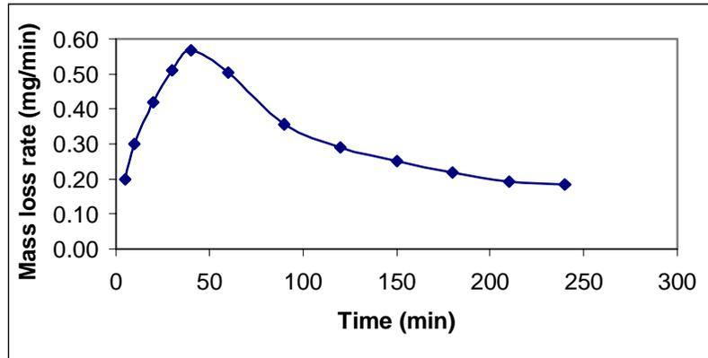
**Figure 2: Mass loss rate for Aluminum sample at 35  $\mu\text{m}$**
