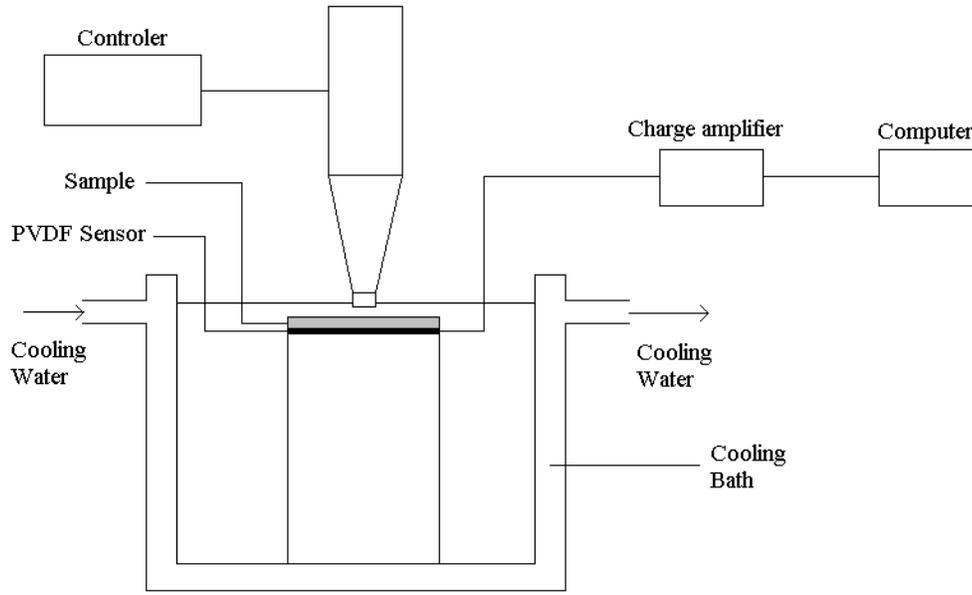
**Figure 1: Schematic of the cavitation test**
