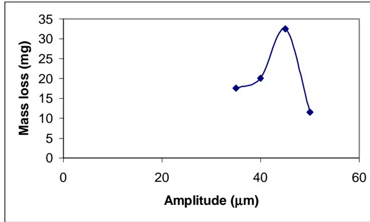
Figure 4: Mass loss after 1-hour exposure tests for the Al sample
