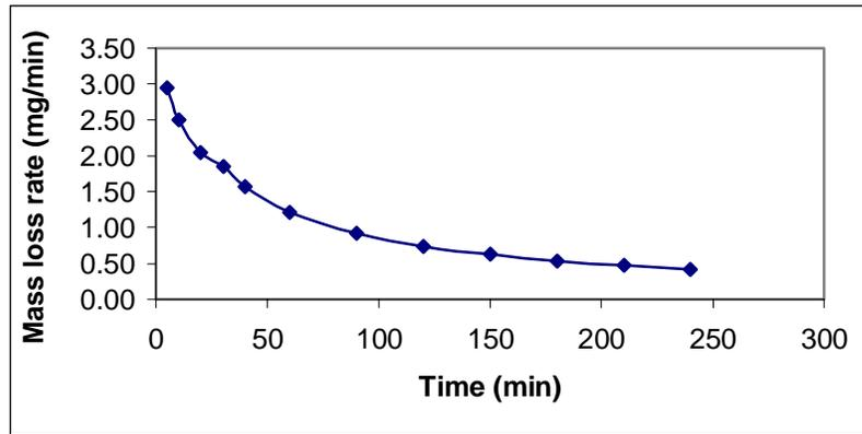
**Figure 3: Mass loss rate for Aluminum sample at 48  $\mu\text{m}$**
