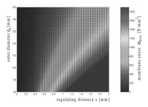
Figure 6- Maximum membrane stress as a function of the outer diameter d<sub>A</sub> and the control distance x.
