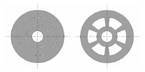
Figure 7- Shapes of membranes with reduced stiffness for higher control distances.
