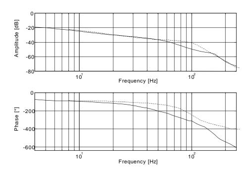
Figure 3- Measured transfer characteristic of the regulating distance for various length of the oil pipes: 2 m (----), 0.5 (---).
