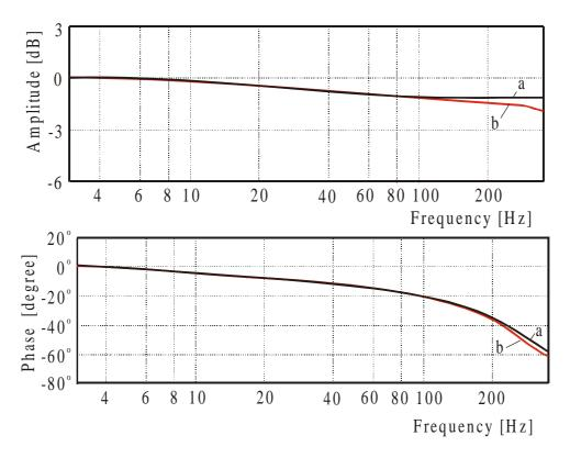
Figure 8- Amplitude and phase response of the magnetic actuators force for two different input currents:  $i(t) = i_s \sin (\omega t)$ ; a)  $i_s = 1,5$  A, b)  $i_s = 3$  A.
