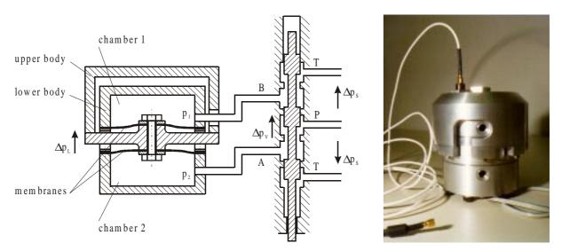
Figure 1- Sketch and prototype of the hydraulic actuator.
