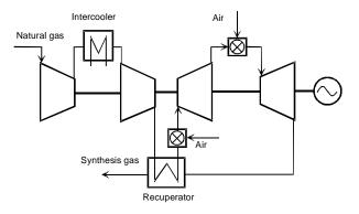
Figure 3 Synthesis gas production in gas turbine system
