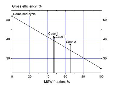
Figure 1 The MSW fraction in the total fuel input versus gross efficiency Gross efficiency Surface area
