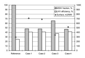
Figure 2 Comparison of the MSW fraction in the total fuel input, the gross plant Efficiency(LHV), and the specific boiler surface area
