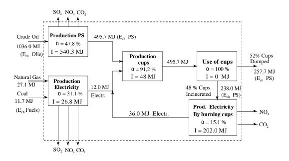
Figure 6 Exergy diagram of the life cycle of the 3000 disposable PS cups
