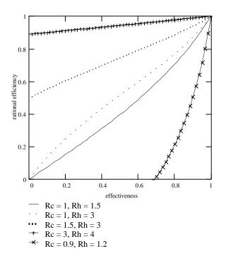
Figure 4: Thermodynamic efficiency versus effectiveness for various cold and hot temperature ratios for  $C_h = C_c$
