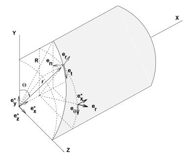
Figure 2: Vectors along Boundary Curve
