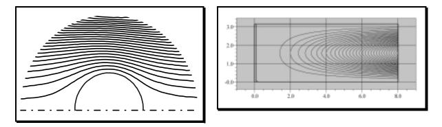
Figure 4 - Visualization of the streamlines external to a gas bubble (cylindrical and spherical coordinates): Re = 10, k = 0.022 and  $\gamma$  = 0.0012.
