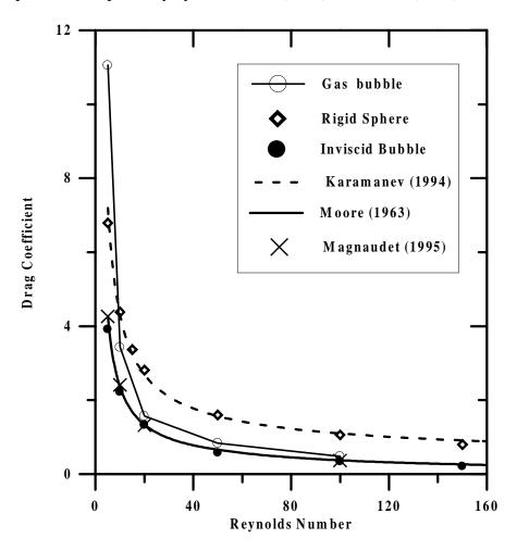
Figure 3 - Gas bubble drag coefficient.
