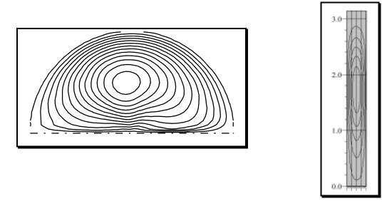
Figure 4 - Visualization of the streamlines inside a gas bubble (cylindrical and spherical coordinates): Re = 10, k = 0.022 and  $\gamma$ = 0.0012.
