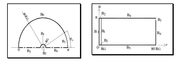
Figure 1 - Flow Domain in cylindrical and spherical coordinates.
