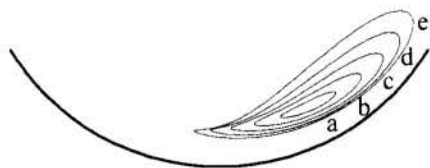
Figure 7: orbits of a shaft journal simulated with the non linear model of a partial arc circular bearing (radius 127 mm, length 127 mm, radial clearance 170 \mu\text{m} , speed 3000 rpm in anti-clockwise direction, static vertical load 10^5 N) at increasing values of the dynamical load (ratio dynamical to statical load = 0.1 (a), 0.2 (b), 0.3 (c), 0.4 (d), 0.5 (e))
