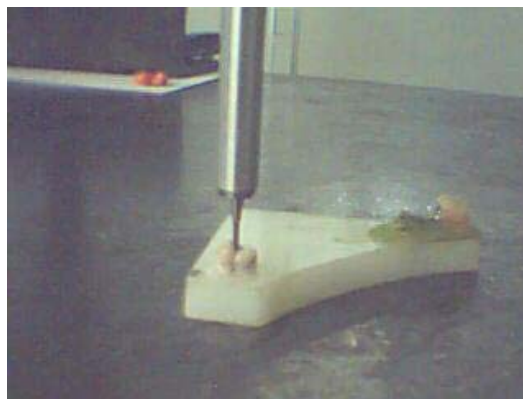
Figure 2 – CMA stylus touching a sample of dental prosthesis
