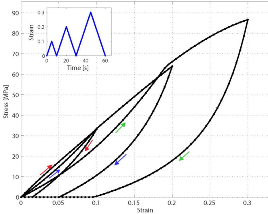
Figure 3: Stress response of the viscoelastic damage fiber contribution
