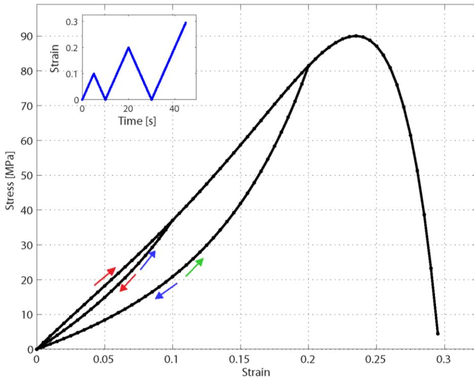
Figure 2: Stress response of the elasto-damage fiber contribution
