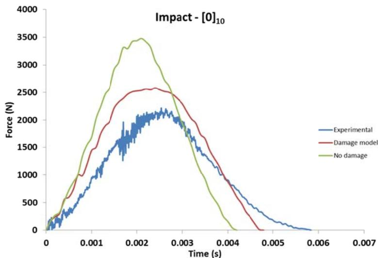
Figure 8: Force vs. Time impact experimental and numerical results for  $[0^{\circ}]_{10}$  laminate.
