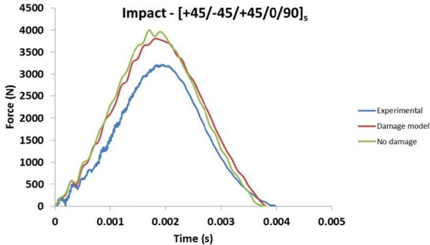
Figure 7: Force vs. Time impact experimental and numerical results for [+45/-45/+45/0/90]<sub>s</sub> laminate.
