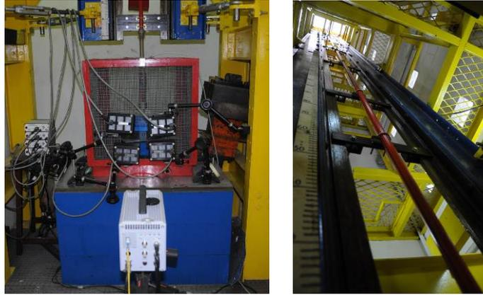
Figure 4: High velocity impact test set up.
