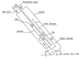
Fig. 1 - Schematic description of the IS-separator, extracted from Ortiz-Vidal et al. (2012)
