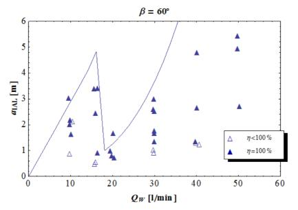
Fig. 3 – Map of efficiency of gas separation as a function of the  $a_{LAL}$  length and of the liquid volumetric flow  $Q_w$  for a 60° inclination angle (solid line). The solid symbols represent total gas separation and the open symbols stand for partial gas separation. The solid line represents the transition boundary predicted by the model.
