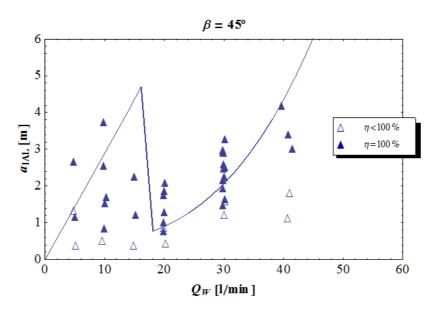
Fig. 2 – Map of efficiency of gas separation as a function of the  $a_{LAL}$  length and of the liquid volumetric flow  $Q_w$  for a 45° inclination angle (solid line). The solid symbols represent total gas separation and the open symbols stand for partial gas separation. The solid line represents the transition boundary predicted by the model.
