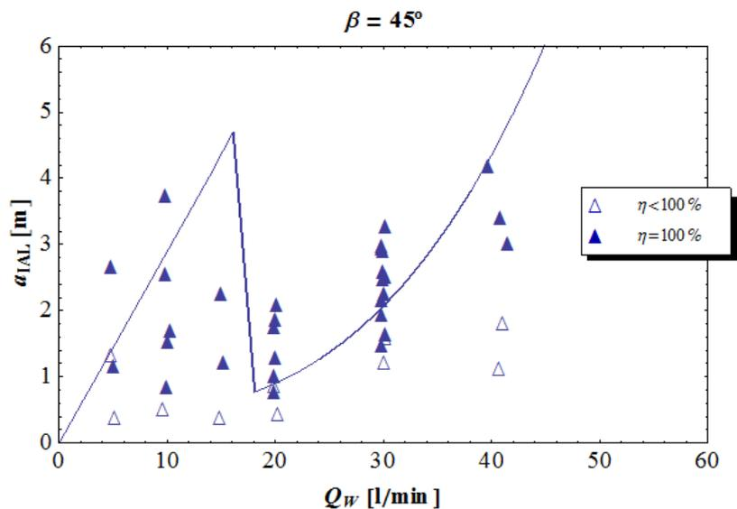
Fig. 2 – Map of efficiency of gas separation as a function of the  $a_{IAL}$  length and of the liquid volumetric flow  $Q_W$  for a 45° inclination angle (solid line). The solid symbols represent total gas separation and the open symbols stand for partial gas separation. The solid line represents the transition boundary predicted by the model.
