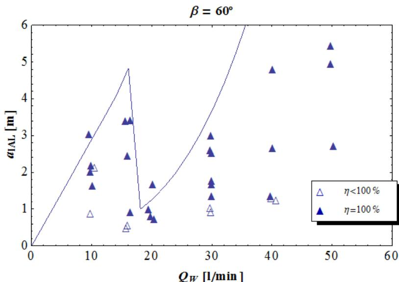
Fig. 3 – Map of efficiency of gas separation as a function of the  $a_{IAL}$  length and of the liquid volumetric flow  $Q_w$  for a  $60^\circ$  inclination angle (solid line). The solid symbols represent total gas separation and the open symbols stand for partial gas separation. The solid line represents the transition boundary predicted by the model.
