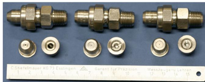
Figure 5: Spray nozzles – Type A (top), B (centre) and C (bottom).
