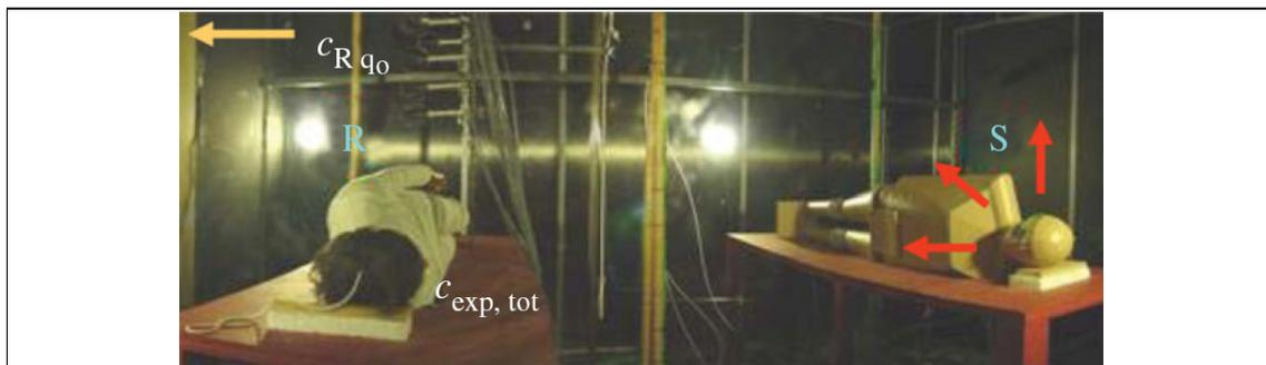
Figure 2 – Dummies simulating two persons laid on hospital beds. The right dummy simulates the infected person, and the other is the target (Nielsen, 2009)
