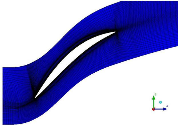
Figure 3. Grid in 70% of span.
