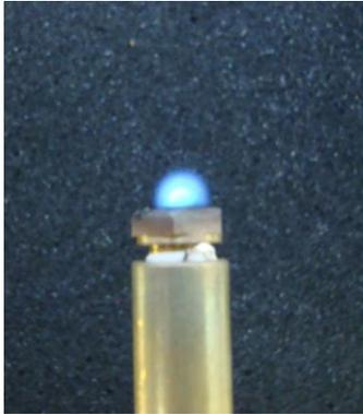
Figure 10. Flame produced with butane and oxygen flow rates  $Q_b = 9,00 \text{ ml/min}$  and  $Q_o = 21,00 \text{ ml/min}$  respectively.
