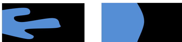
Figure 2. Viscous fingering and plug displacement, respectively
