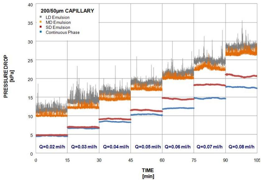
Figure 5. Evolution of the pressure drop as the flow rate varies for the continuous phase and emulsions. Flow rate range:  $Q = 0.02 - 0.08 \text{ ml/h}$ . Capillary diameter:  $200 \mu\text{m}$ . Constriction diameter:  $50 \mu\text{m}$ .
