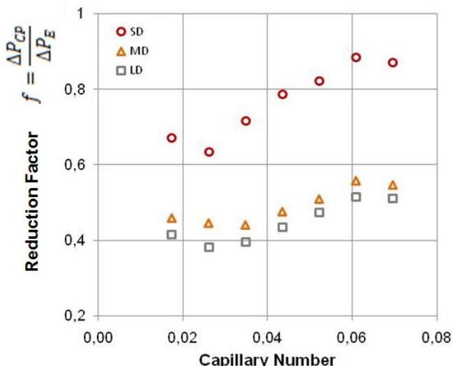
Figure 8. Reduction factor as a function of the Capillary number for the injected emulsions through the 100/50 $\mu$ m capillary.
