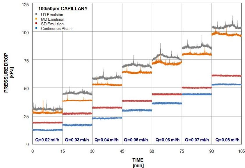
Figure 4. Evolution of the pressure drop as the flow rate varies for the continuous phase and emulsions. Flow rate range:  $Q = 0.02 - 0.08$ ml/h. Capillary diameter: 100µm. Constriction diameter: 50µm.
