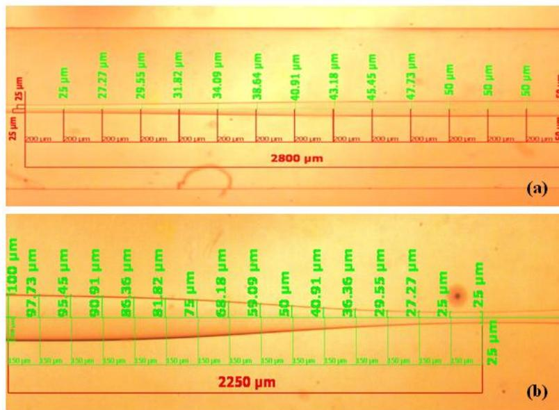
Figure 2. Photographs of the 100/50µm (a) and 200/50µm (b) constricted capillaries.
