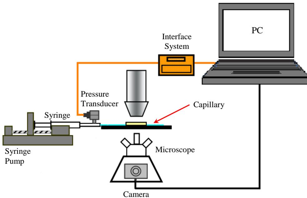
Figure 3. Experimental setup used to measure pressure drop as a function of time.
