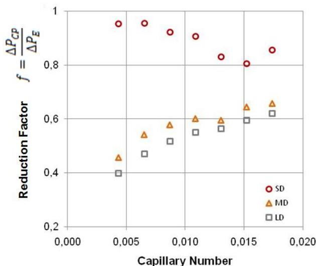
Figure 9. Reduction factor as a function of the Capillary number for the injected emulsions through the 200/50 $\mu$ m capillary.
