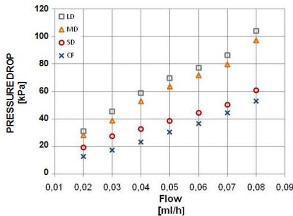
Figure 6. Average pressure drop-flow rate relation for the  $100/50 \mu\text{m}$  capillary.
