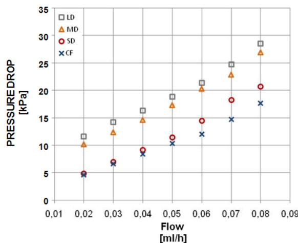
Figure 7. Average pressure drop-flow rate relation for the  $200/50 \mu\text{m}$  capillary.
