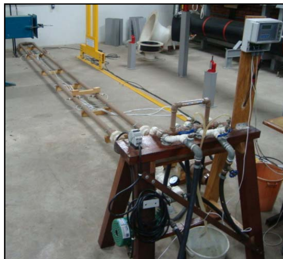
Figure 1 – (a) Pipe prover basic scheme and main parts; (b) pipe prover assembled at laboratory
