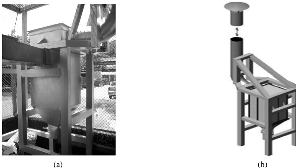
Figure 4 - (a) shows the collection system and filtering the flue gas and (b) Shows the design used for their construction of it. Source: Akel, 2008
