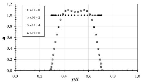
Figure 3. Dimensionless temperature profile for Pr = 1 and  $Re_D = 100$ .
