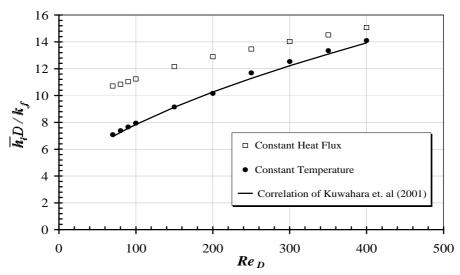
Figure 6. Effect of  $Re_D$  on  $h_i$  for Pr = 1.
