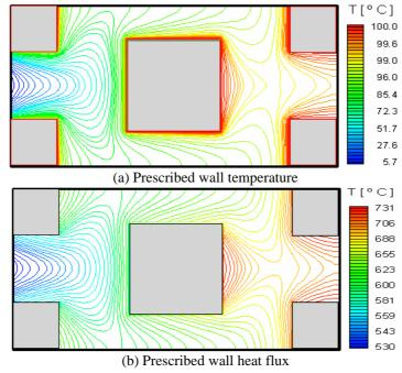
Figure 4. Isotherms for Pr = 1 and  $Re_D = 10$ .
