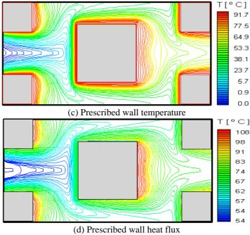
Figure 5. Isotherms for Pr = 1 and  $Re_D = 100$ .
