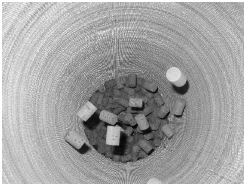
Figure 3. The spouted bed of cork stoppers viewed from above. The stoppers are kept in a bag made with a stainless steel mesh to ease particles introduction and extraction from the bed.
