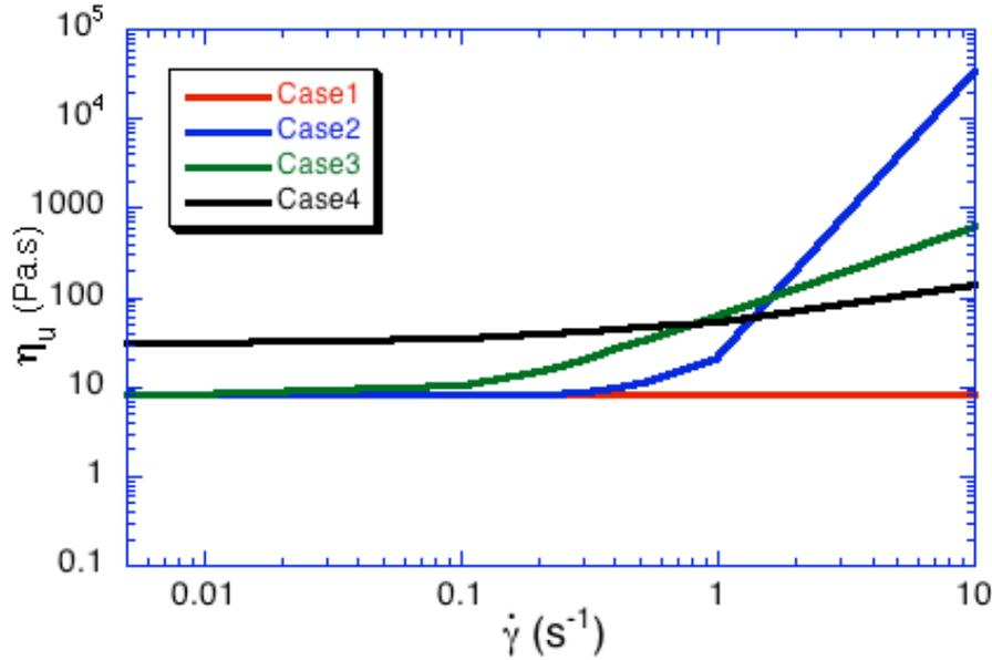
Figure 2: The extensional viscosity function,  $\eta_u$ .
