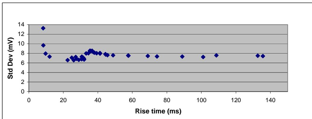
Figure 5: Standard deviation as a function of number of rise time data points for 500 psi (34,5 bar)
