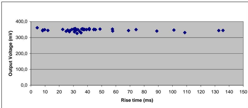
Figure 4: Output voltage as a function of rise time por 500 psi (34,5 bar)
