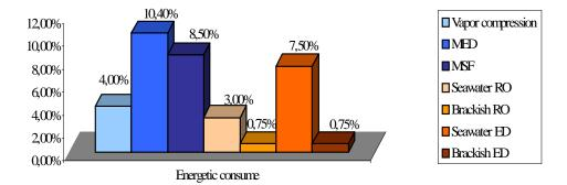
Figure 4 – Energetic consume (kg oil/m<sup>3</sup> of purified water)
