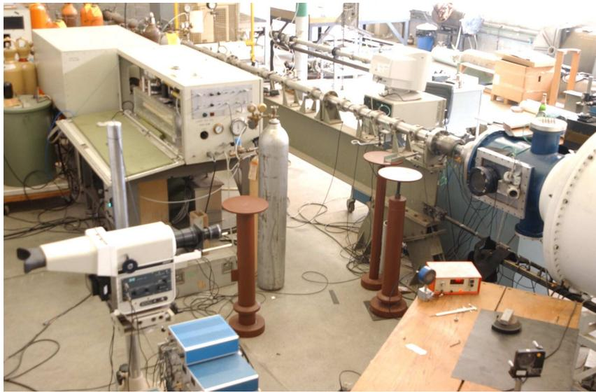
**Figure 3. HST test section and the CO<sub>2</sub> TEA laser heads.**
