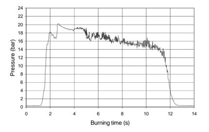
Figure 5: Motor chamber pressure (test 1).
