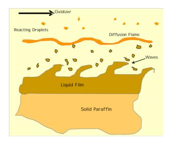
Figure 1: Thin-film instability of paraffin based solid fuel under oxidation (adapted from Dornhein, 2003).
