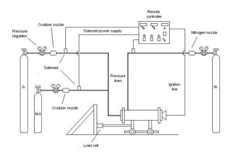
Figure 2: Test stand for hybrid rockets.
