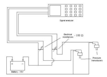
Figure 4: Data acquisition schematic.
