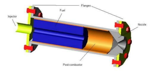
Figure 3: Hybrid motor assembly.
