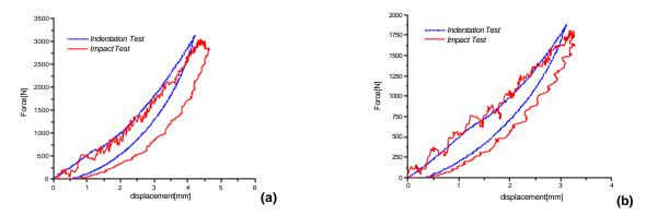
Figure 15 - Results for laminate [0/90/0/90/0]s: (a) maximum force at 3,000 N; (b) maximum force at 1,750 N
