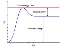
Figure 3 – Impact Energy, Absorbed Energy e Elastic Energy
