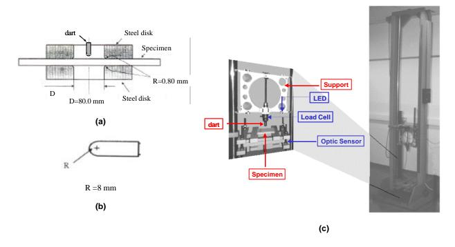
Figure 5 – (a) Composite plates clamped by two circular steel disks; (b) Geometry of the dart; (c) Drop tower at LCPC of Katholieke Universiteit Leuven (Belgium)
