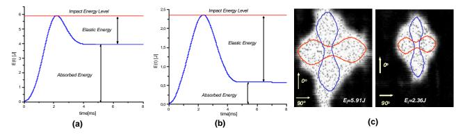
Figure 10 – Results for laminate [0/90/0/90/0]<sub>s</sub>: (a) energy-time for 5.91 J; (b) energy-time for 2.36 J; (c) Results for laminate [0/90/0/90/0]<sub>s</sub>: C-Scan images
