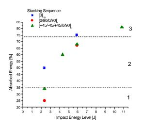
**Region 3**: the specimens show many type of failure mechanics, for example: fiber rupture, matrix crack and delaminations; so, the fraction of absorbed energy is very high (over 75%)
