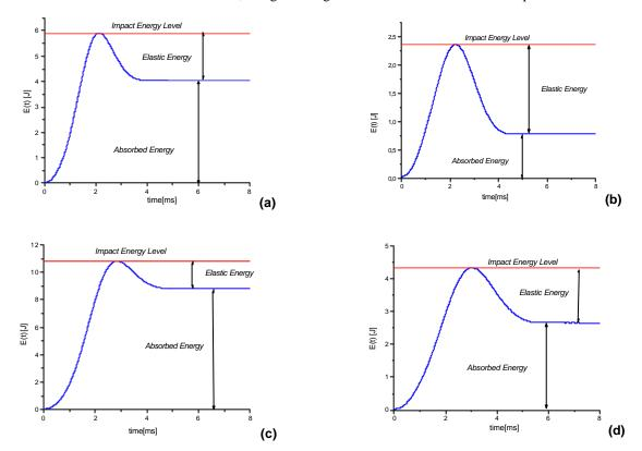
Figure 12 – Results for laminate [+45/-45/+45/0/90]₅: (a) energy-time for 5.91 J; (b) energy-time for 2.36 J; (c) energy-time for 10.82 J J; (d) energy-time for 4.33 J
