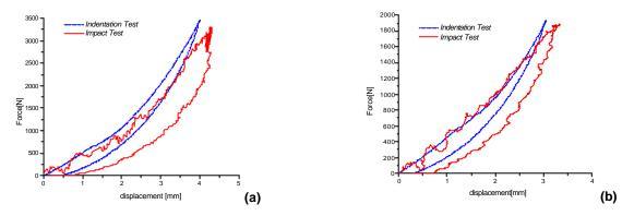
Figure 16 – Results for laminate [+45/-45/+45/0/90]s: (a) maximum force at 3,300 N; (b) maximum force at 1,900 N
