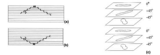
Figure 2 – Delaminated plies: (a) Thick laminate ("pine tree"); (b) Thin laminate ("reverse pine tree"); (c) "Peanut shapes" (Abrate, 1998)
