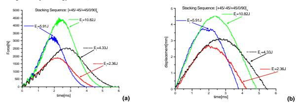
Figure 11 – Results for laminate [+45/-45/+45/0/90]s: (a) force-time; (b) displacement-time
