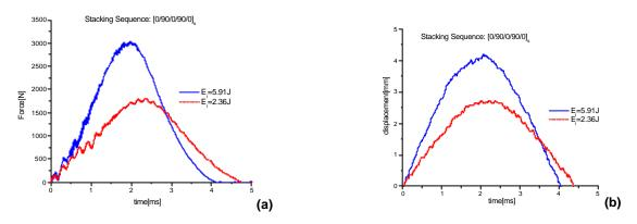
Figure 9 – Results for laminate [0/90/0/90/0]s: (a) force-time; (b) displacement-time
