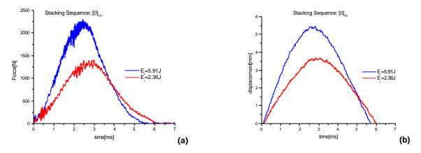
Figure 7 – Results for laminate [0]10: (a) force-time; (b) displacement-time
