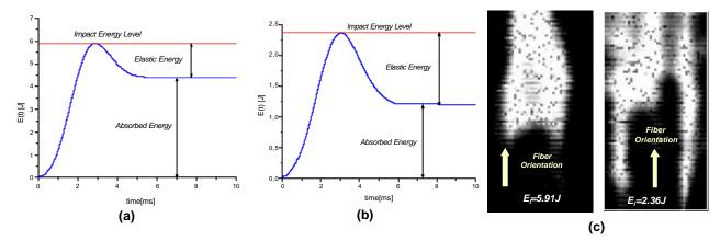
Figure 8 – Results for laminate [0]<sub>10</sub>: (a) energy-time for 5.91 J; (b) energy-time for 2.36 J; (c) Results for laminate [0]<sub>10</sub>: C-Scan images
