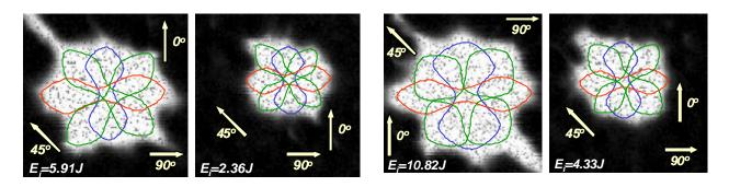
Figure 13 - Results for laminate [+45/-45/+45/0/90]s: C-Scan images
