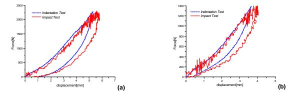
Figure 14 – Results for laminate [0]<sub>10</sub>: (a) maximum force at 2,250 N; (b) maximum force at 1,300 N
