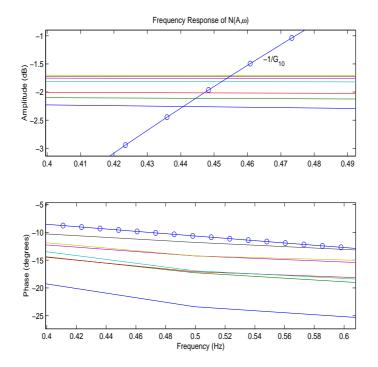
Figure 7 – Frequency response of the nonlinear hydraulic actuator and the inverse of the  $G_{10}$  system.
