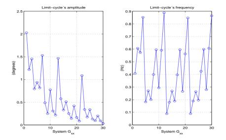
Figure 3 – Frequency and amplitude of the limit cycle for each closed loop experiment.
