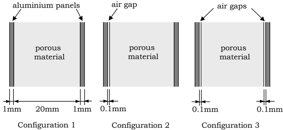
Figure 3 – Configurations for double panel lining
