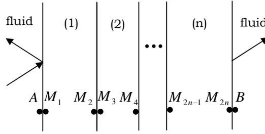
Figure 2 – Sound transmission through multilayered system
