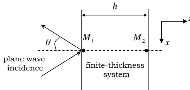
Figure 1 – Plane wave impinging upon finite-thickness system
