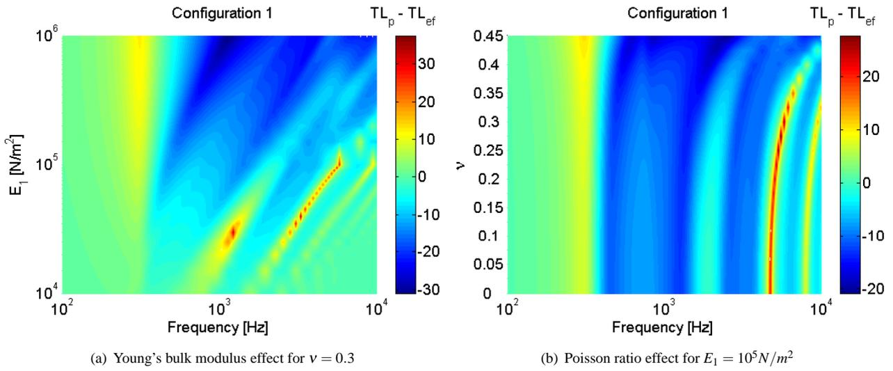
Figure 4 – Difference in the  $TL$  of the models for configuration 1
