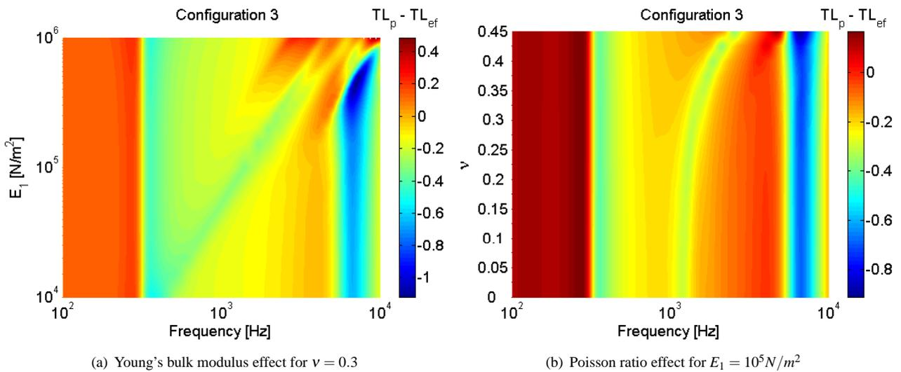
Figure 6 – Difference in the  $TL$  of the models for configuration 3
