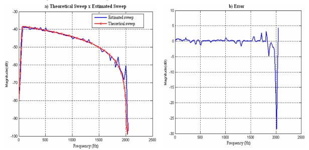
Figure 10: a) Comparison between theoretical and estimated sweep at receiver point. b) Error (theoretical sweep minus estimated sweep).
