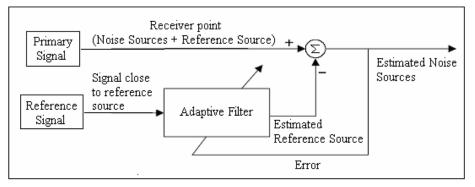
Figure 1 – Scheme of adaptive filter
