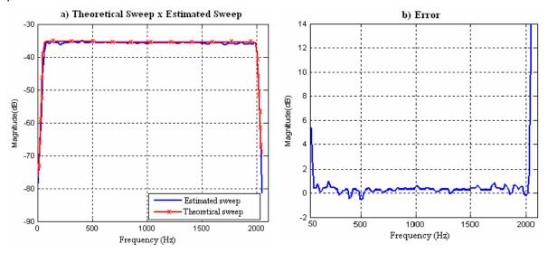
Figure 6: a) Comparison between theoretical and estimated sweep at receiver point. b) Error of theoretical sweep in relation to estimated sweep.
