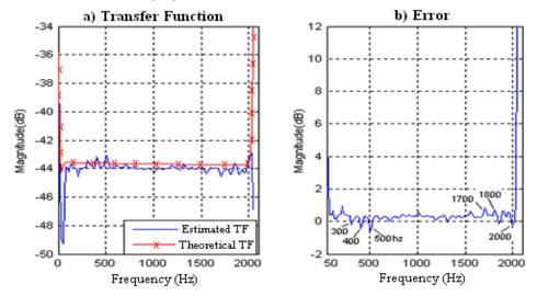
Figure 8: a-Spectral density power of the estimated transfer function and the theoretical transfer function. b- Error of the theoretical transfer function.
