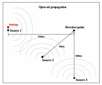
Figure 4 – Simulation model with three noise sources
