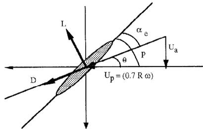
Figure 6 Propeller forces in function of the angle of attack.
