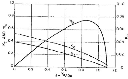
Figure 4  $k_T$  and  $k_Q$  hydrodynamic coefficients.
