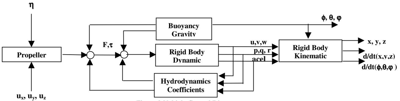
Figure 9 Vehicle Control Diagram.
