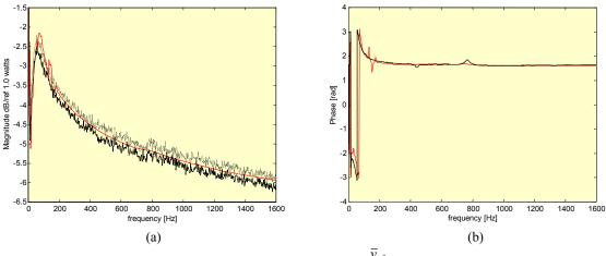
Figure 9: Source mobility: (a) magnitude and (b) phase: ---  $\overline{Y}_S = \frac{\overline{v}_{sf}}{\overline{f}_{bl}}$ , -- "direct method", --- "mass method"
