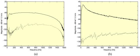
Figure 3: Source velocity with:(a) periodic CHIRP signal and (b) RANDOM signal under: - FREE and --- BLOCKED conditions
