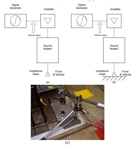
Figure 1: Experimental Setup: (a) FREE condition; (b) BLOCKED condition; (c) PLATE receptor
