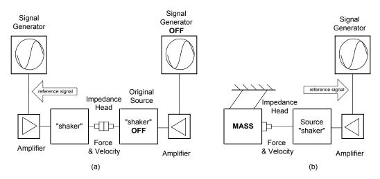
Figure 8: Experimental Setup of Source Mobility: (a) "direct method"; (b) "mass method"
