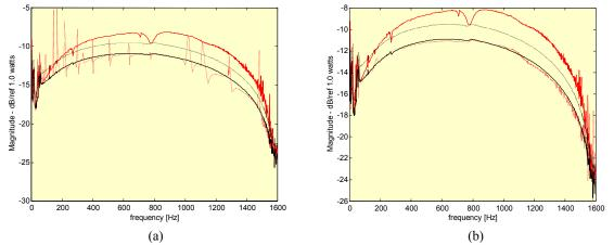
Figure 6: Power terms for the BEAM with:(a) LIGHT damping and (b) HEAVY damping; source with periodic CHIRP signal: ---  $|\overline{Q}|$  input power, --- |MAP|, --- |MP|, --- |CP|
