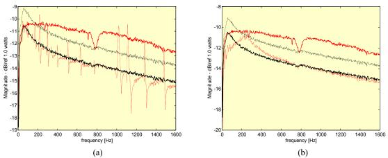
Figure 7: Power terms for the BEAM with:(a) LIGHT damping and (b) HEAVY damping; source with RANDOM
