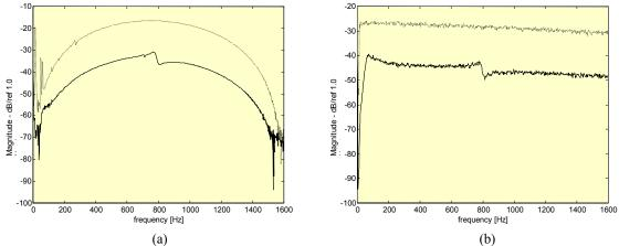
Figure 2: Source force with:(a) periodic CHIRP signal and (b) RANDOM signal under: - FREE and --- BLOCKED conditions
