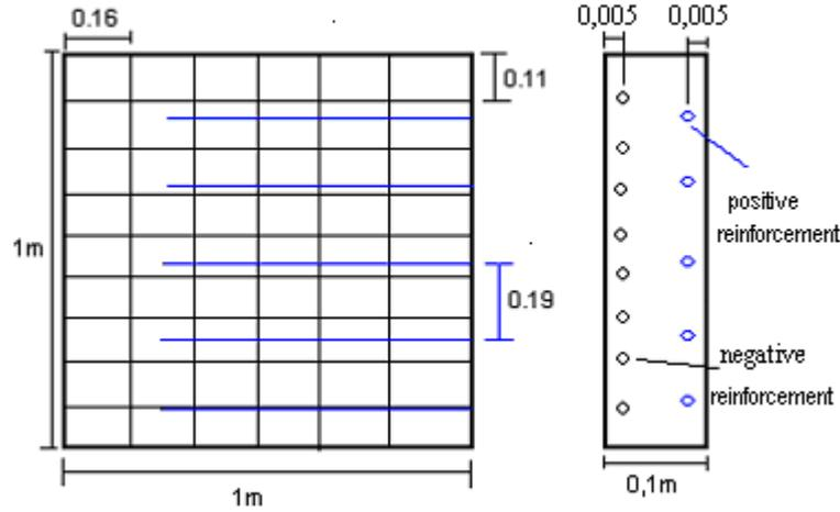
Figure 1 - Reinforced concrete flagstone
