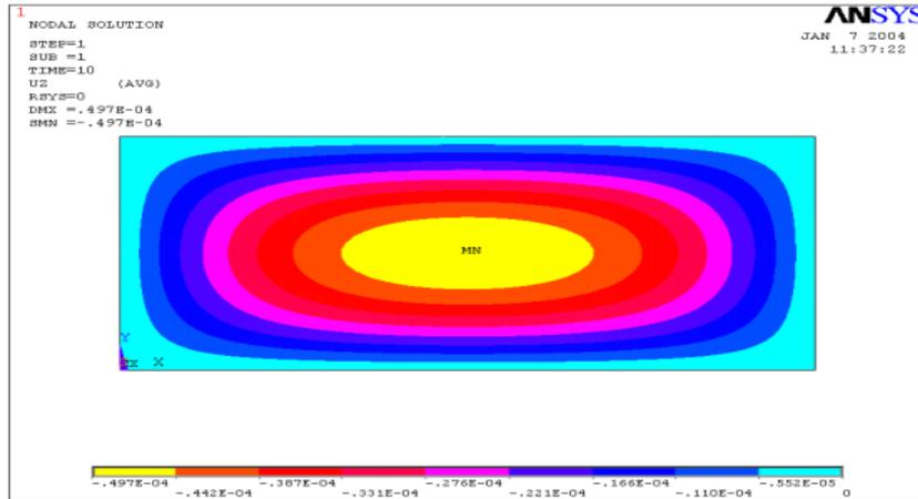
Figure 6 - Area 1 modeled with 'Shell93' and equivalent Modulus of Elasticity given by Eq.1
