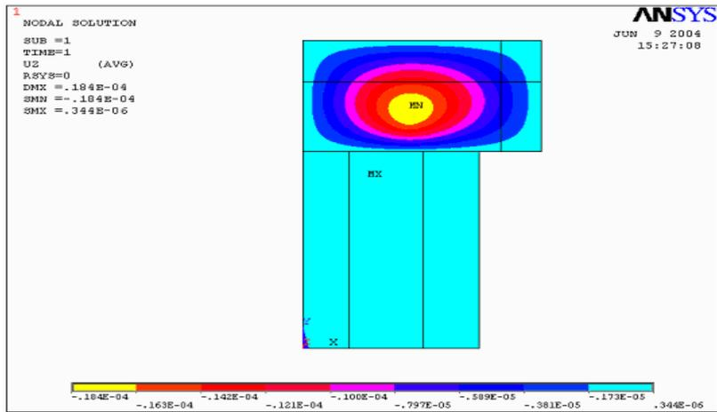
Figure 9 - Displacement obtained in the structure at t=1s.
