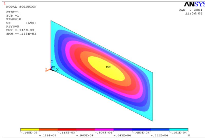
Figure 5 - Area 1 modeled as element 'Shell93'
