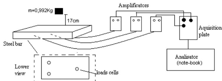
Figure 3 - Experimental workbench utilized for determination of the impact force.
