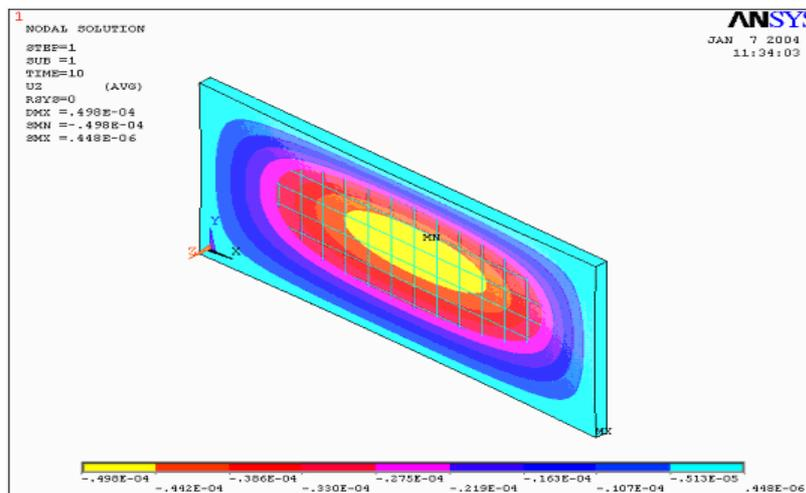
Figure 4 - Area 1 modeled as element 'Solid65'
