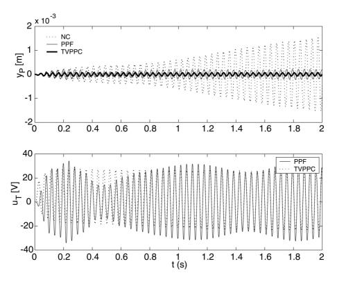
Figure 7. Time response of the system without control and controlled as the temperature goes from 4.4° C to 37.7° C.
