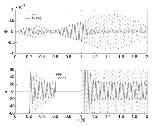
Figure 9. Failure effect / delay simulation of the controller, with saturation, at variable temperature.
