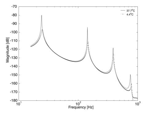
Figure 2. Frequency response function at 4.4 °C and 37.7 °C.
