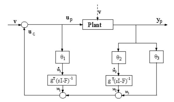
Figure 4. State-space realization of TVPPC; v as a command signal (solid line) or as an unknown disturbance to the plant (dashed line).
