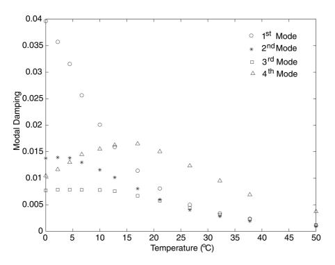
Figure 3. Modal damping versus temperature.
