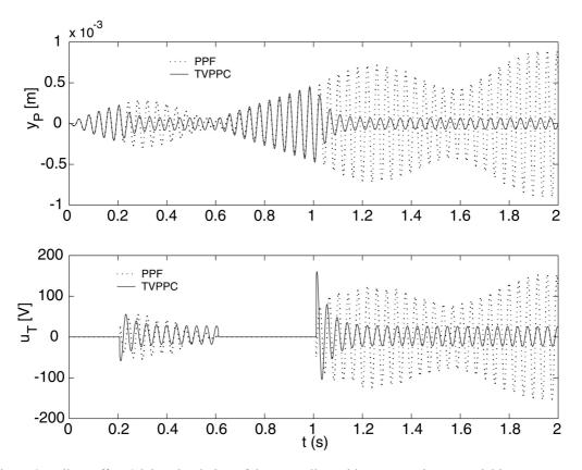
Figure 8. Failure effect / delay simulation of the controller, without saturation, at variable temperature.
