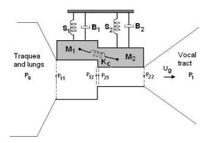
Figure 4. Mechanical model for the vocal cords, proposed by Flanagan and Ishizaka (1972).
