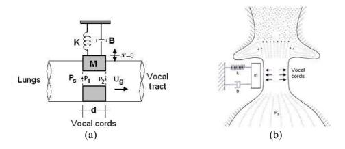
Figure 3. (a) Mechanical model for the vocal cords; (b) Vocal system used (adapted from Titze (1980)). (Flanagan and Landgraf model (1968)).
