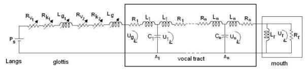
Figure 5. The acoustic circuit representation proposed by Flanagan and Ishizaka (1972).
