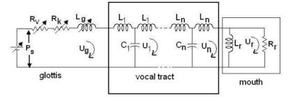
Figure 2. Acoustic circuit representation for the production of voiced sounds.
