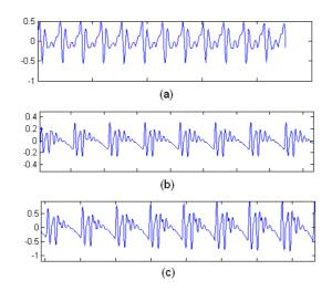
Figure 8. Comparison of signals: (a) real voice signal, vowel /a/ sustained; (b) and (c) synthetic voice signal
