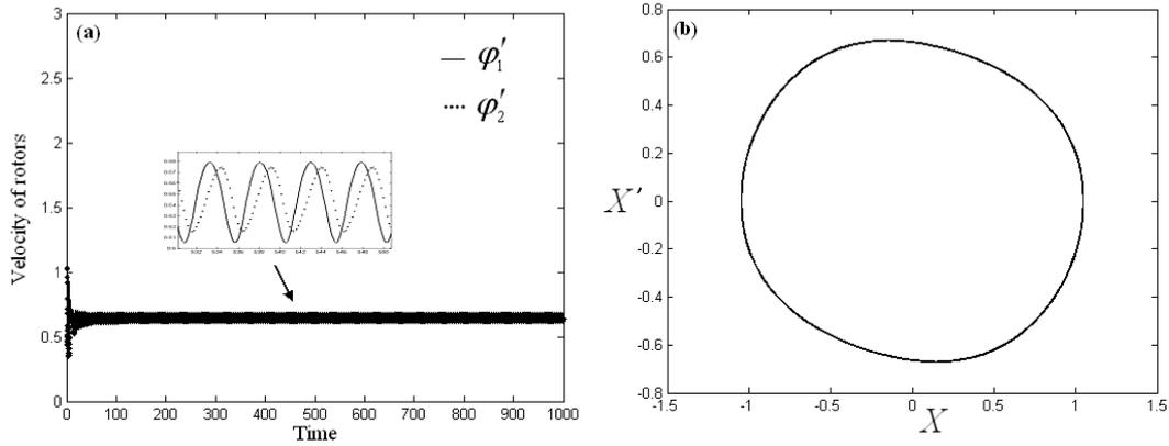
Figure 3. a) Velocity of rotors and b) phase plane for  $\hat{a}_1 = 1.0$  and  $\hat{a}_2 = 0.93$ : self-synchronization.
