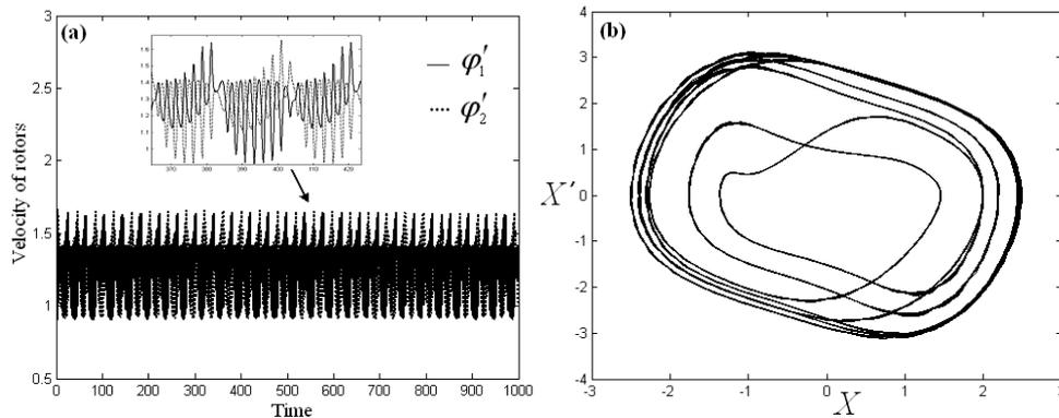
Figure 4. a) Velocity of rotors and b) phase plane for  $\hat{a}_1 = 2.0$  and  $\hat{a}_2 = 2.005$ : absence of self-synchronization.
