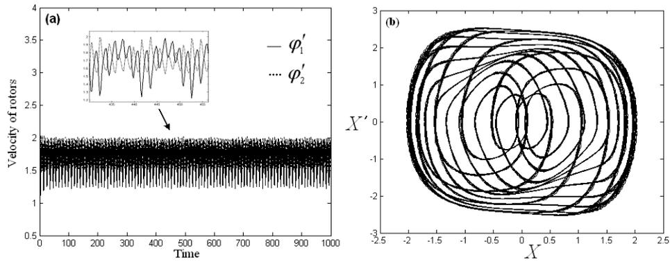
Figure 5. a) Velocity of rotors and b) phase plane for  $\hat{a}_1 = 3.0$  and  $\hat{a}_2 = 2.2$ : absence of self-synchronization.
