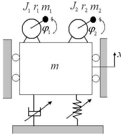
Figure 1. Non-ideal nonlinear and self-excited system model
