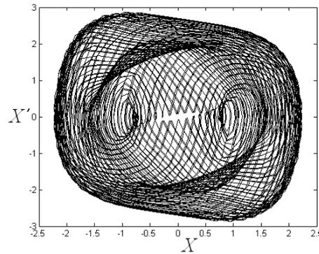
Figure 6. Phase plane plot for  $\hat{a}_1 = 3$  and  $\hat{a}_2 \in [2.3, 2.5]$ : absence of self-synchronization and chaotic motion.
