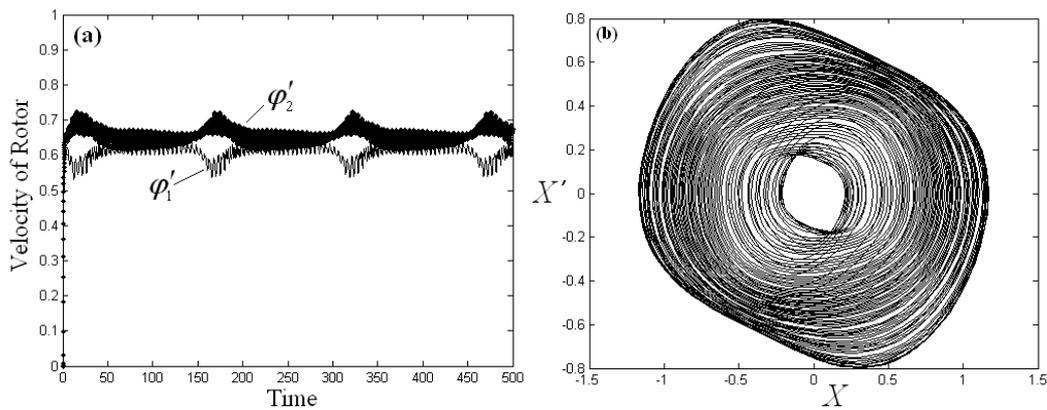
Figure 2. a) Velocity of rotors, b) phase plane for  $\hat{a}_1 = 1$  and  $\hat{a}_2 = 0.9$ : self-synchronization by intervals.
