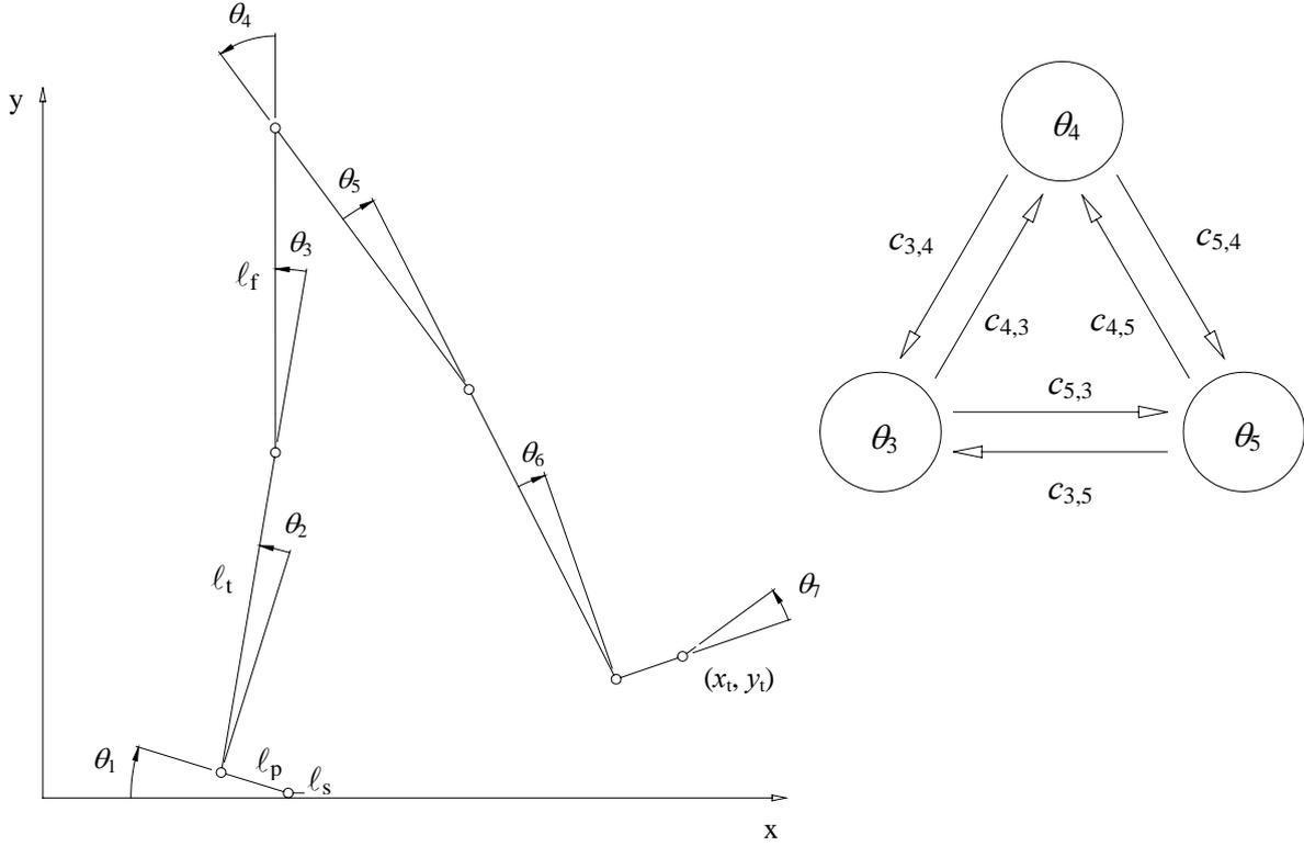
Figure 2. Model of the bipedal robot to be analyzed and structure of coupling between the oscillators.
