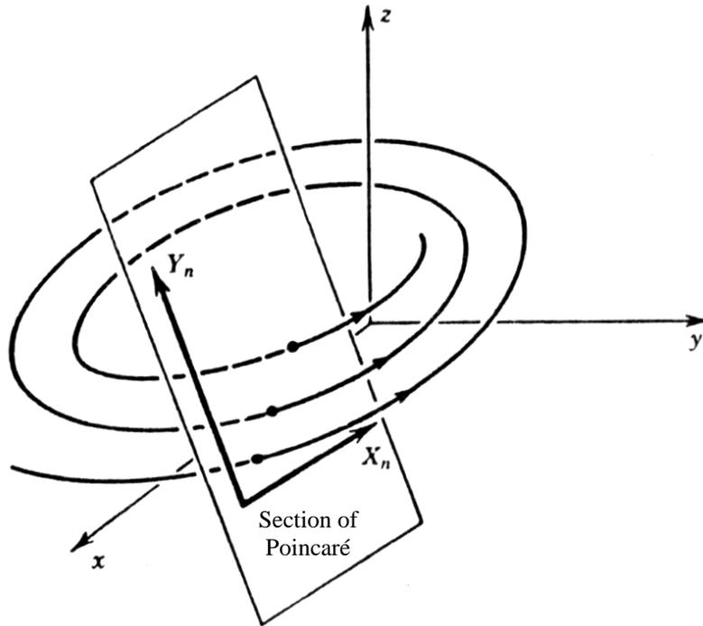
Figure 4. Section of Poincaré in a three-dimensional phase space (Moon, 1998).
