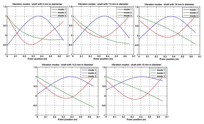
Figure 2. Mode shapes as a function of the rotor flexibility
