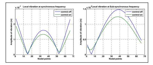
Figure 6. Vibration along of rotor before and after control - shaft with 10 mm in diameter (case E)
