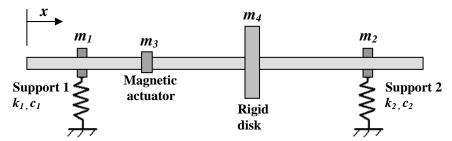
Figure 1. Sketch of rotor for analysis of active control of vibration with magnetic actuator
