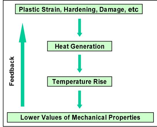
Figure 1. Thermomechanical coupling in metallic elements subjected to inelastic strain loadings.
