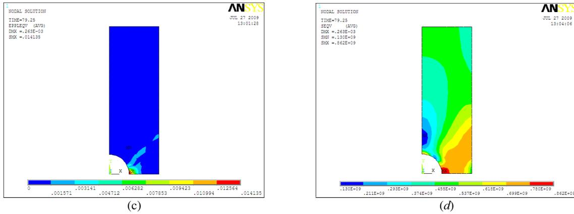
Figure 3. Equivalent plastic strain distribution (a) and von Mises equivalent stress distribution (b). *Uncoupled model*. Equivalent plastic strain distribution (c) and von Mises equivalent stress distribution (d). *Coupled model*.
