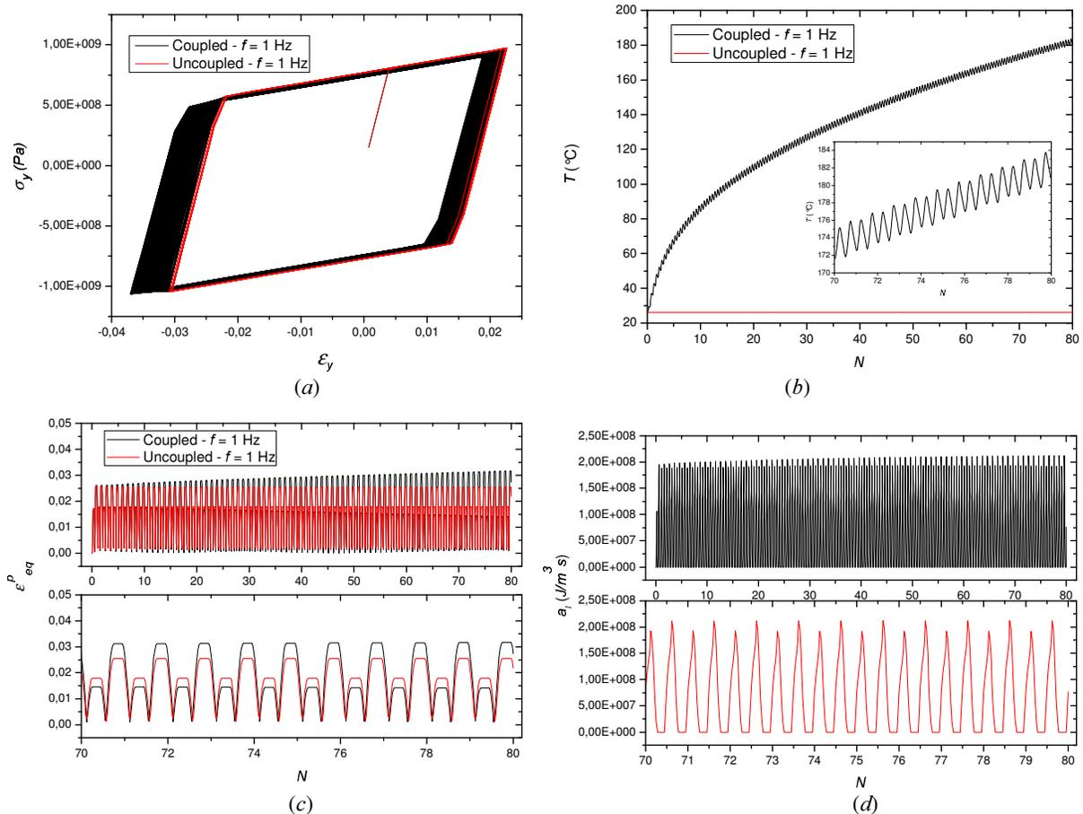
Figure 4. Stress-strain curve (a). Temperature (b), equivalent plastic strain (c) and the internal coupling term (d) evolution.
