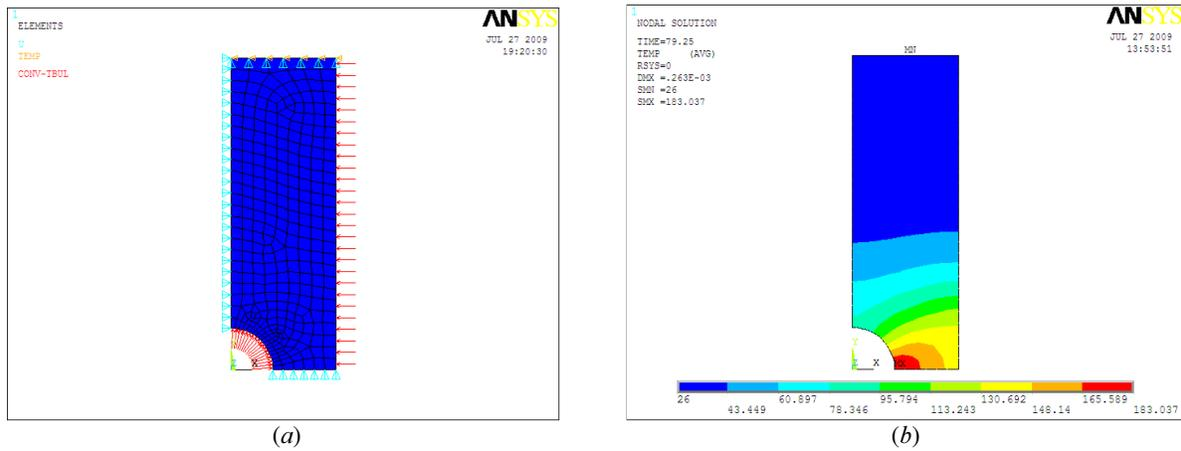
Figure 2. Mesh with boundary conditions and loadings (a) and temperature distribution for the *coupled model*.
