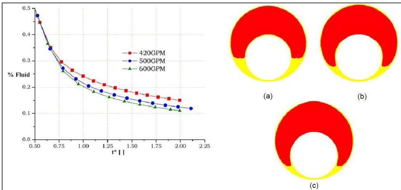
Figure 10. Completion fluid displacing (red) drill-in fluid (yellow) in horizontal 8 1/2" – 5" annulus, fully eccentric, for different pump rates, cross section in the middle of the geometry, Pump rates – (a) 0,0265 m<sup>3</sup>s<sup>-1</sup> (420 gpm), (b) 0,0315 m<sup>3</sup>s<sup>-1</sup> (500 gpm) and (c) 0,0378 m<sup>3</sup>s<sup>-1</sup> (600 gpm).
