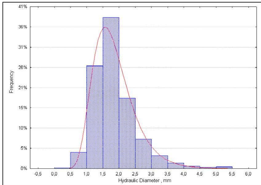
**Figure 6. Chart Lognormal for hydraulic diameter of cuttings obtained for a well of Espirito Santo basin.**
