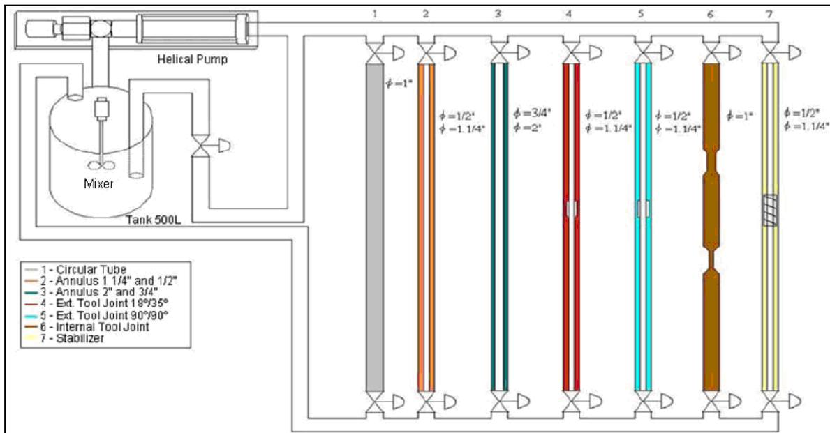
Figure 3. Scheme of experimental unit of fluids flows.
