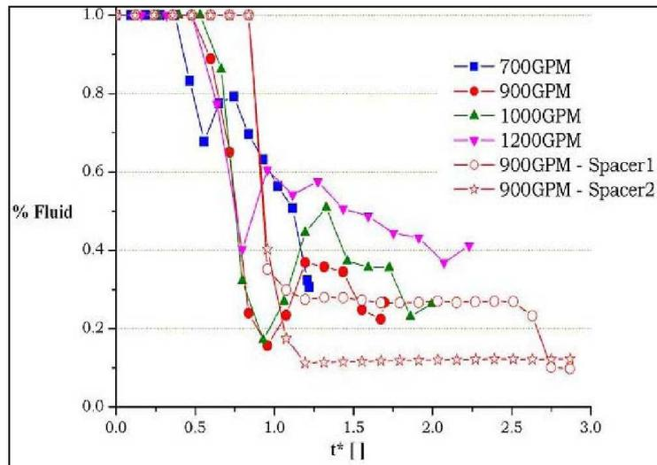
Figure 9. Chemical wash displacing a synthetic fluid in a riser.
