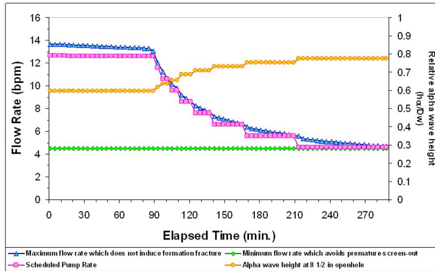
Figure 11. Variable Pump rate schedule.
