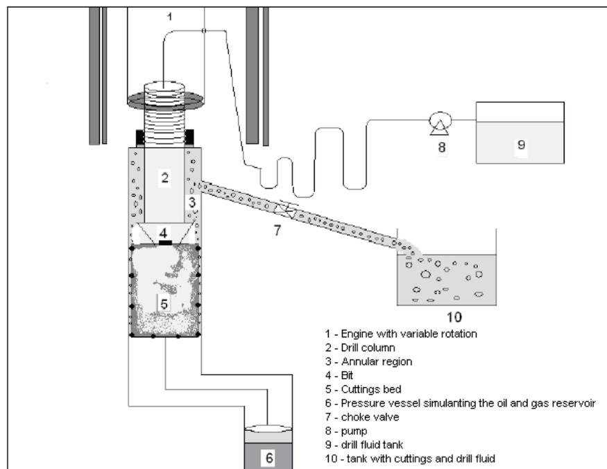
Figure 4. Scheme of experimental unit for pressure control in drill operations.
