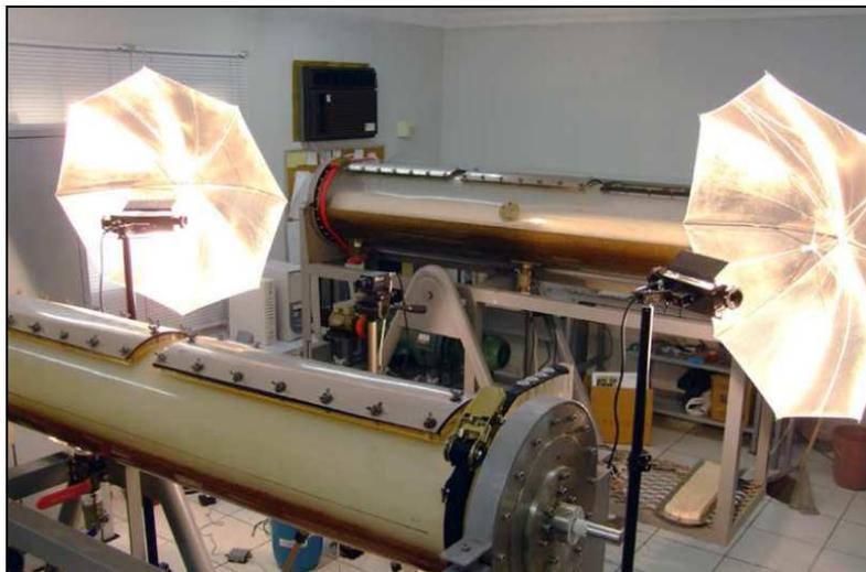
**Figure 7. Experimental apparatus for study of re-suspension of cuttings bed in horizontal wells.**
