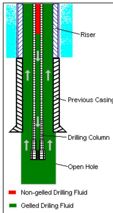
**Figure 5. Restart of the circulation of drilling fluid.**
