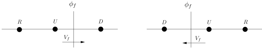
Figure 1. Position of compute nodes D , U and R according to the sign of V_f speed of a convective variable \phi_f .
