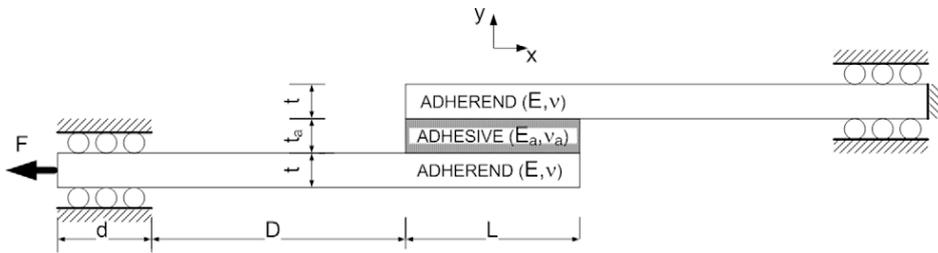
Figure 1. Simple shear condition.
