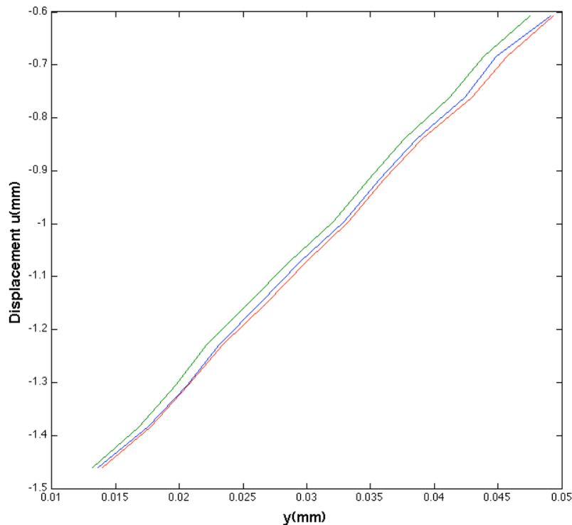
Figure 5. Horizontal displacement curves for applied load of 80 N, for different temperatures.
