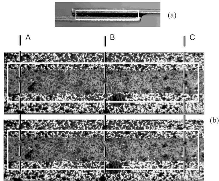
Figure 4. Single lap joint in the overlap: (a) analysis region and (b) pattern of the coating specimen.
