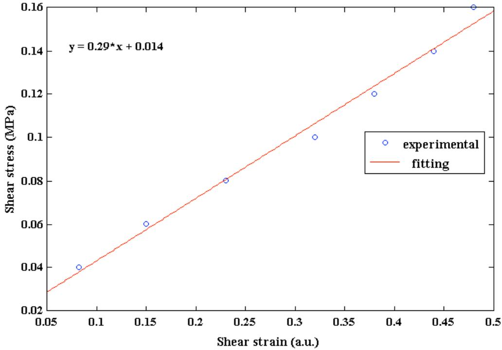
Figure 6. Stress x strain curve for different applied loads, for the temperature of 50 °C.
