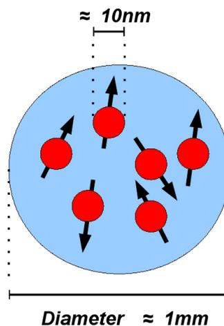
Figure 1. Sketch of the geometry: a fuel droplet with embedded magnetic nanoparticles.
