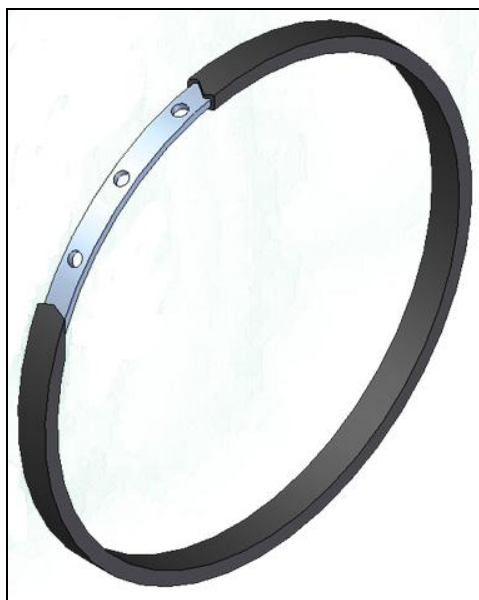
Figure 11. Plastic lined steel ring.
