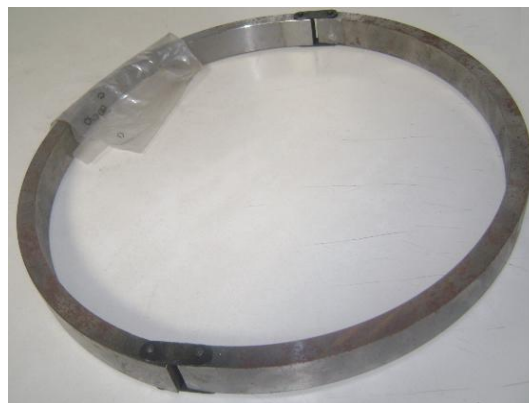
Figure 7. Split steel ring.
