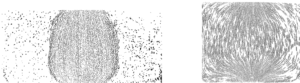
Figure 6: Experimental streamlines for the viscoplastic liquid \alpha_0^0 = 0.14; L/D = 0.5 and 1
